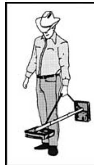
Figure 6. Handle strap: Using the handle strap increases depth; however, it may be difficult to tune the GEMINI-3 this close to highly mineralized ground.
