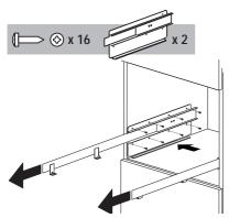
Position the rails on the sides of the cabinet as shown in the figure. Fix with the screws, then extract them completely. If the coffee maker is installed over a warmer drawer, use the top surface of this as a reference to position the rails. In this case, there will be no surface to rest the rails on.
