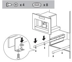
Position the appliance on the rails, making sure the pins are correctly inserted in the housings, then fix it with the screws supplied.
