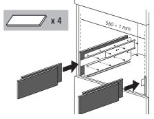
If necessary, correct alignment of the appliance by positioning the spacers supplied under or at the sides of the support.
