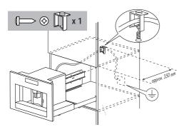
Fix the power cable with the clip. The power cable must be long enough to allow the appliance to be extracted from the cabinet to fill the coffee bean container.
