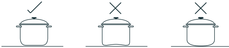
Fig.11 Use cookware with flat and smooth bases to provide good contact with the glass
