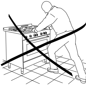
Fig. 17 Incorrectly moving the cooker
