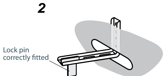
Fig. 3c Fitting the lock pin through the bracket
