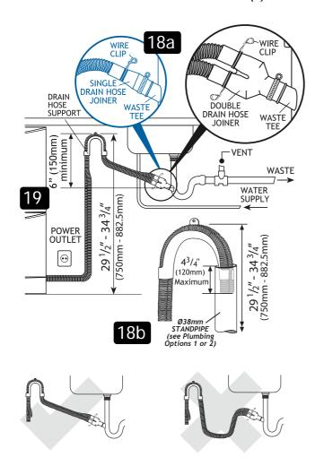
DishDrawer® with Hose Joiner (see Plumbing Options). Remember to slip the wire clip(s) on the drain hose(s) first.
