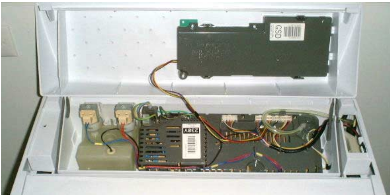
PHASE 5 TOPDECK SHOWING WIRING CONNECTIONS
