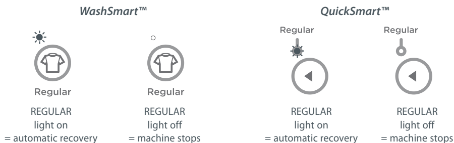
Fig.38 Adjusting the Out of balance recovery routine
