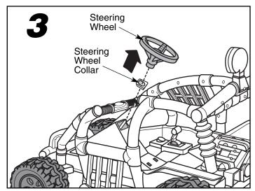
Remove the steering wheel and steering wheel collar from the old steering column.
