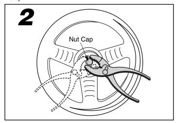
**Note:** When removing the cap nut from the old steering column, you will crush it. We have included a new cap nut in this kit for re-assembly.
