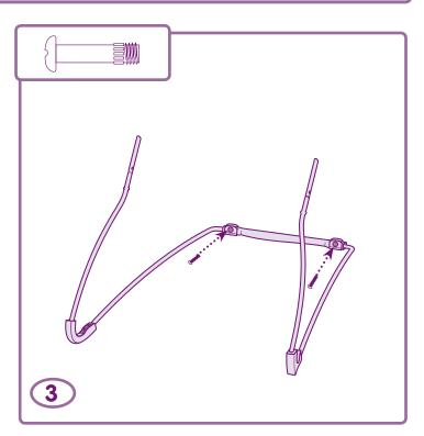
• Insert an M5 x 20 mm screw through each foot and tighten.
