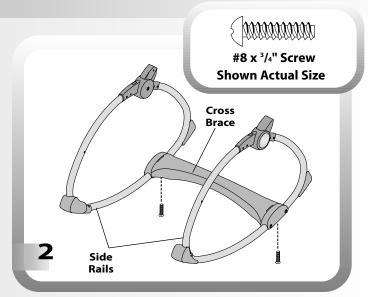
Insert a screw through the hole in the bottom of each side rail and into the cross brace. Tighten the screws with a Phillips screwdriver. Do not over-tighten.
