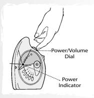
Place receiver in room in which you intend to use it. Rotate the power/volume dial to turn power on. Power indicator lights. Adjust receiver location.
