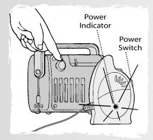
Place transmitter in room in which you intend to use it. Rotate transmitter power switch to turn power on. Power indicator lights. Turn on a radio.
