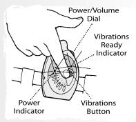
Clip receiver to your clothing (where you will feel vibrations). Walk to the furthest point of use. Rotate receiver power/volume dial to turn power on. Power indicator lights. Now, press the vibrations button. Vibrations ready indicator lights.
