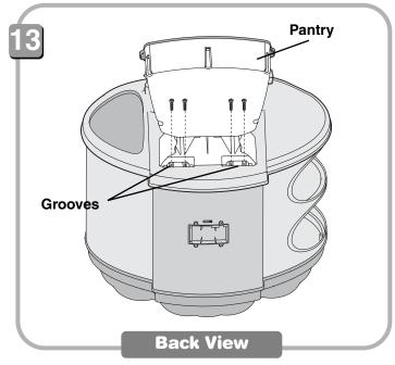
Insert four screws through the grooves in the pantry and into the counter top. Tighten the screws with a Phillips screwdriver. Do not over-tighten.
