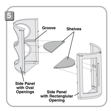
Slide each shelf into the groove in each side panel.
