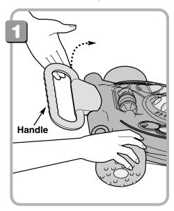
• While holding one of the rear wheels, lift the handle.
