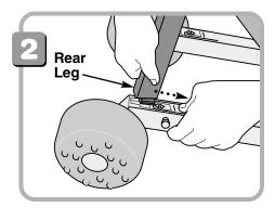
While pressing the arrow, carefully slide the rear leg slightly toward the front wheel.
