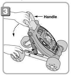
While holding one of the rear wheels, push the handle down toward the rear wheels until it "snaps" into place.
