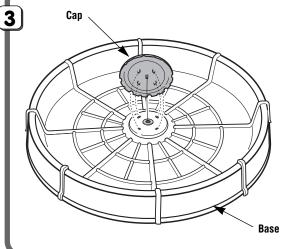
• Insert and snap the cap to the base and panels. **Assembly is now complete.**
