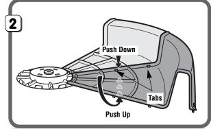
Helpful Hint: You may have difficulty snapping the panel tab closest to the base. Lift the assembly up slightly. While pushing up from the underside of the assembly (directly below the tab), push down on the topside of the assembly (directly above the tab).
