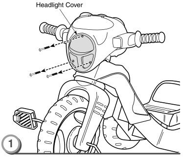
Loosen and remove the screws from the headlight cover.
