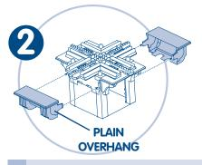
"Snap" the plain overhangs into the base, as shown.
