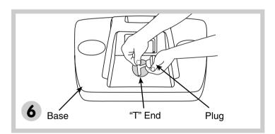
Bend the "T" end of the plug and insert it into the hole in the base.
