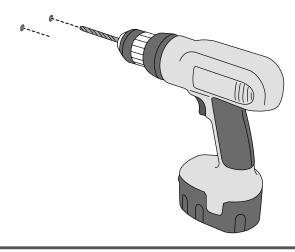
• Using a ¼" drill bit, drill one hole through each pencil mark you made on the wall.
