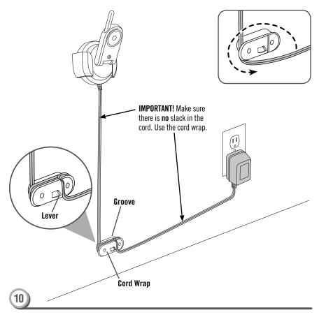
**IMPORTANT!** Make sure the cord is taught between the camera docking station and cord wrap. Excess cord can form loops or extend into the crib and present a strangulation hazard.
