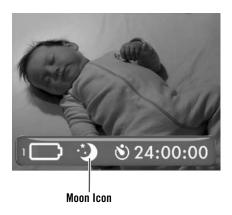
When the light in baby's room is too low, the camera will automatically switch to night vision mode. The moon icon will appear on the menu bar, and the image on the video screen will appear in black and white, not color.
