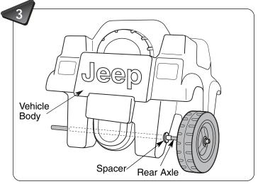
• Insert the rear axle through the holes in the rear of the vehicle body. Make sure the spacer fits into the hole in the vehicle body.
