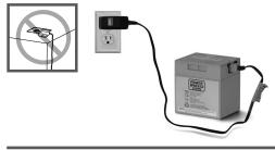
· Plug the charger into a standard wall outlet.
