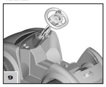
• While carefully feeding the wire down into the dash, fit the steering wheel onto the end of the steering column.
