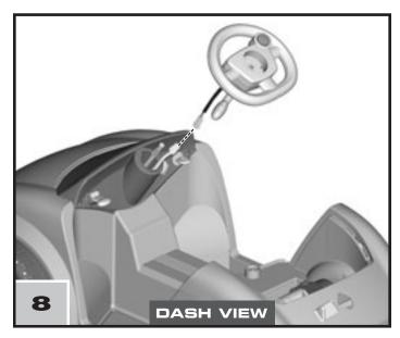
• Plug the motor harness connector from the vehicle into the steering wheel connector.
