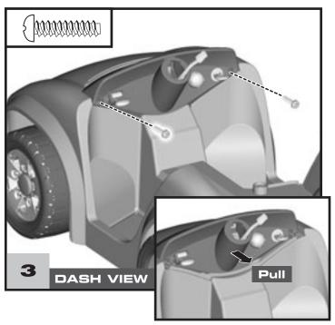
• Insert two #8 x  $^{3}\!\!\!/\!\!\!4$ " screws straight into the dash, as shown. Tighten the screws.
