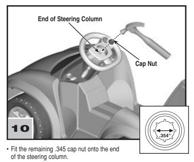
• Tap the cap nut with a hammer to secure it to the end of the steering column.
