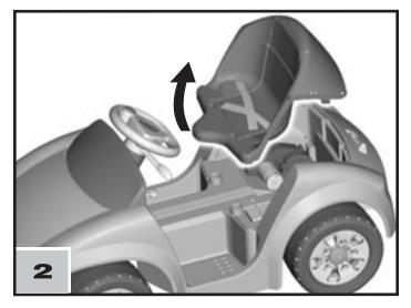
Grasp under the front of the seat and lift firmly to remove it.
