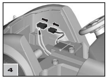
• Plug the battery connector into the motor harness connector.
