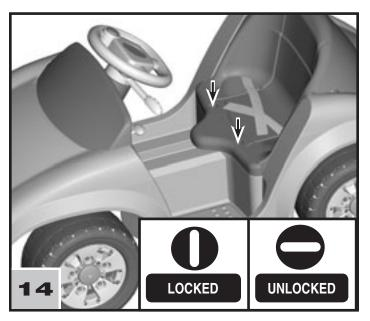
Using a slotted screwdriver, turn both lock fasteners ¼ turn to the locked position ①.
