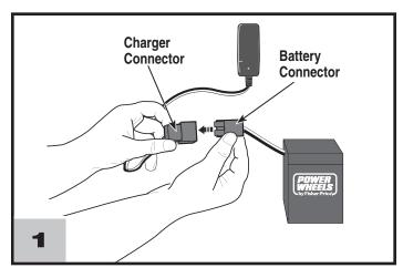
Plug the battery connector into the charger connector.
