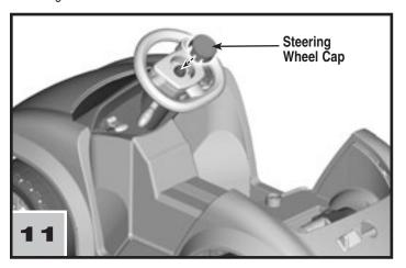
• "Snap" the steering wheel cap into the center of the steering wheel.
