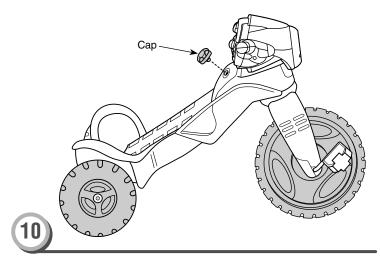
• Insert and "snap" the cap into the hole in the frame.
