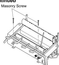
Figure 12 - Attaching Base Assembly to Fireplace Floor
