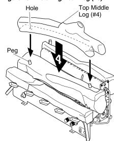
Figure 20 - Installing Crossover Log (#4)
