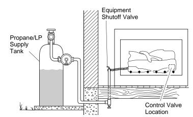
Figure 16 - Checking Gas Joints
