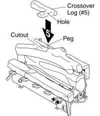
Figure 21 - Installing Crossover Log (#5)
