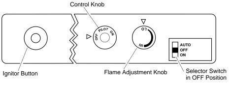
Figure 22 - Control Knob and Ignitor Button Location
