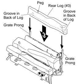
Figure 19 - Installing Rear Log (#3)
