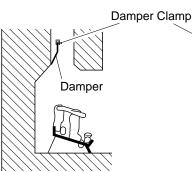
Masonry Fireplace Manuf Figure 10 - Attaching Damper Clamp
