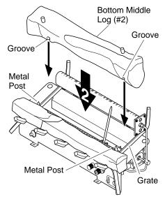
Figure 18 - Installing Bottom Middle Log (#2)
