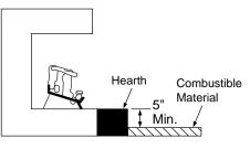
Figure 9 - Minimum Fireplace Clearances Above Combustible Flooring
