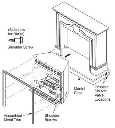
Figure 12 - Installing Fireplace without Flange
