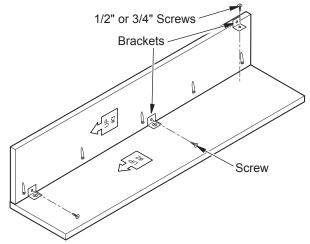
Figure 2 - Attaching Brackets
