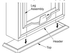
Figure 5 - Placing Mantel Assembly onto Mantel Top
