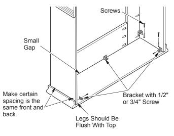
Figure 6 - Attaching Top to Leg and Header Assembly
