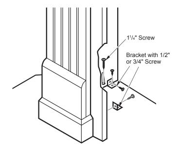
Figure 9 - Installing Brackets to Mantel Base
