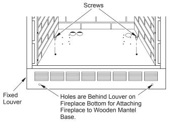
Figure 11 - Screw Locations for Fireplaces with Fixed Louver
