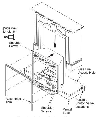
Figure 8 - Installing Fireplace with Flange
