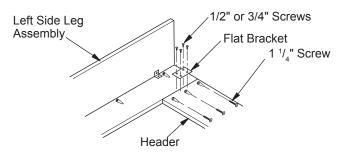
Figure 4 - Attaching Header to Leg Assembly
