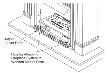
Figure 10 - Attaching Fireplace to Mantel and Mantel Base
