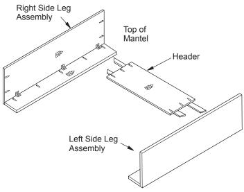
Figure 3 - Installing Header
