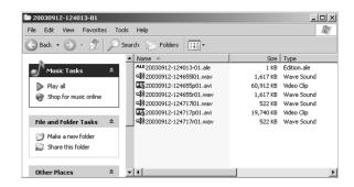
Once clips have been imported into Liquid Edition, an Index file is created on the disk drive per clip. Do not delete this file since it is required to continue work in the particular project. The illustration below shows this.
