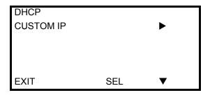
With the IP settings menu item, you can select either DHCP (the network provides the IP address) or a CUSTOM IP.
