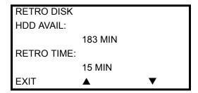
◆ Set RETRO TIME by pressing the ▲ and ▼ buttons. Time is selectable in one minute increments.
