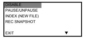
◆ DISABLE - This selection allows you to connect a 3.5mm to DB9 cable to the GPI port and control the FS-2/2E using RS232C from an external device. You can also use the FS-2/2E with the optional wired remote control unit (ACSS-0019-01). Purchase this item at the Focus Enhancements online store: https://www.focusinfo.com/sales/store/.
