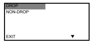
This selection is not applicable for PAL use. On the FS-2/2E display, DROP is identified by a semicolon (;) and NON-DROP by a colon (:).
