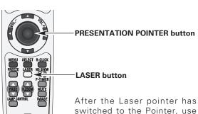
After the Laser pointer has switched to the Pointer, use the LASER button as the Pointer function ON-OFF switch. Press the LASER button toward the projector and see if it lights green.
