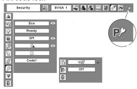
When the projector is locked with the PIN code, the PIN code lock mark appears on the menu bar.
