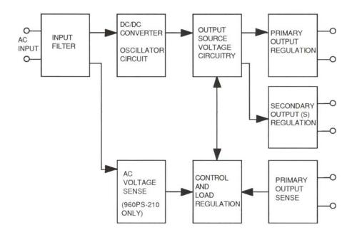
Figure 1-1. Power Supply Functional Block Diagram
