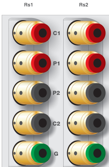
Figure 5 External Resistor Inputs
