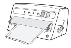
4. After red light goes off, rotate latch to unlock, lift door and remove bag (Fig. 3).
