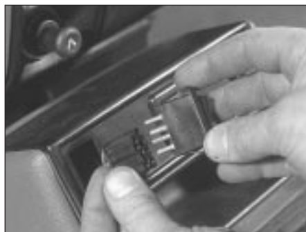
4.20b . . . then disconnect its multiplug and remove the switch
