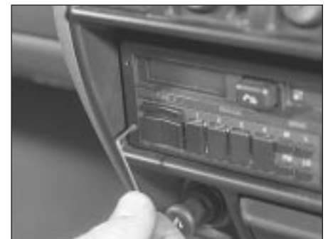
22.2 Unscrewing the securing pins from the radio/cassette player
