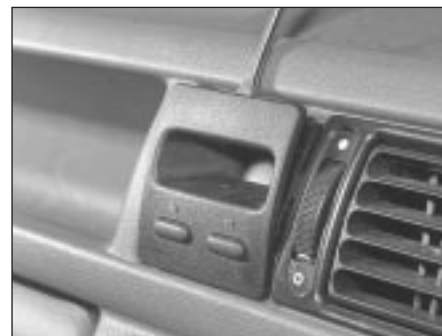
13.2 Carefully prise the clock out of the facia
