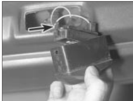
5.29 Release the number plate light securing tab (arrowed) and separate the bulbholder and light cover
