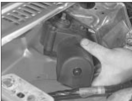
16.8b . . . and withdraw the wiper motor assembly
