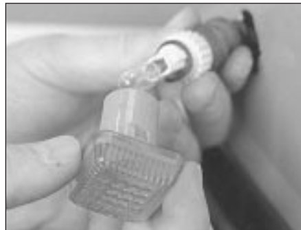
5.13 Removing the direction indicator side repeater bulbholder assembly
