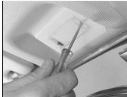
6.16a Releasing the interior (courtesy) light from its location
