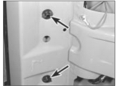
5.24a On Courier models, unscrew the two black plastic nuts securing the rear light cluster assembly . . .
