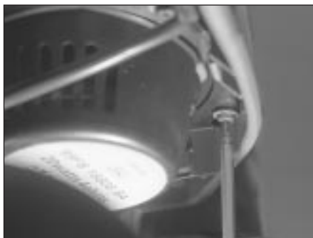
23.5a Remove the rear speaker securing screws . . .
