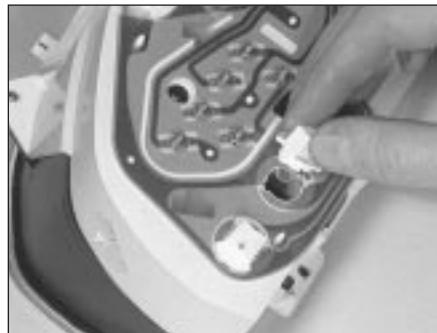
10.2 Removing a bulbholder from the rear of the instrument cluster (bayonet type fitting)
