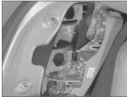
5.21b . . . then having pressed its retaining lugs, withdraw the bulbholder for access to the bulbs
