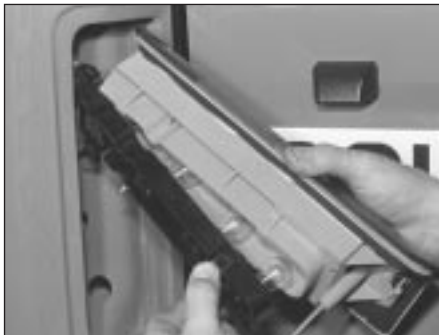
5.24b . . . then withdraw the assembly to the outside of the vehicle
