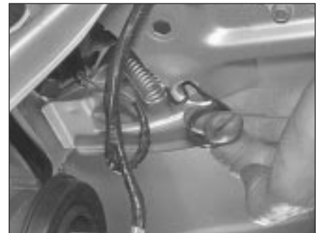
7.7a Release the front direction indicator light retaining spring from its body location . . .
