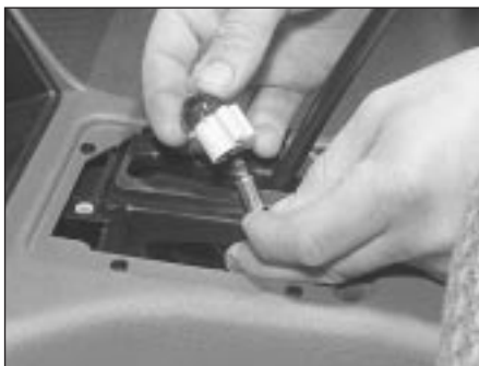
6.3a Remove the selector illumination bulb cover . . .
