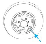
Inspect the tire side walls for cuts, bruises and other damage. If internal damage to the tire is suspected, have the tire demounted and inspected in case it needs to be repaired or replaced.
