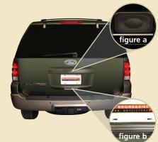
To open the liftgate glass, push the button (figure a) under the center of the license plate
