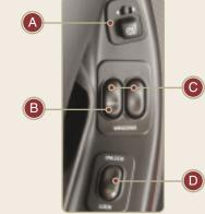
A Power Side View Mirrors (if equipped) -Move the selector control to the left to adjust the left mirror, or to the right to adjust the right mirror. Next, move the mirror control in the direction you wish to tilt the mirror. Return the selector control to the center position to lock the mirrors in place.
