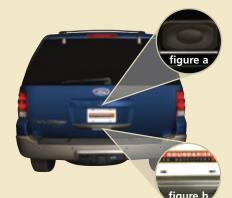
To lower the liftgate glass, push the button (figure a) under the center of the license plate
