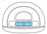
With the ignition key in the ACC or ON position, the rear dome lamp can be turned ON or OFF by sliding the control.
