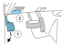
The BRAKE warning lamp will illuminate and will remain illuminated until the parking brake is released.
