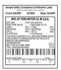
Exceeding the Safety Certification Label vehicle weight rating limits could result in substandard vehicle handling or performance, engine, transmission and/or structural damage, serious damage to the vehicle, loss of control and personal injury.
