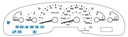
Make sure the corresponding lights illuminate or illuminate briefly. If a light fails to illuminate, have the vehicle serviced.
