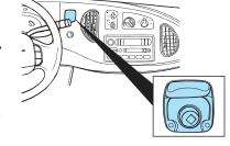
The auxiliary power point is located on the instrument panel.
