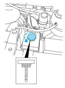
Check the fluid level when it is at ambient temperature,  $20^{\circ}$  –  $80^{\circ}$  F (-7° –  $25^{\circ}$  C):
