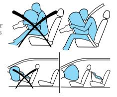
All occupants of the vehicle, including the driver, should always properly wear their safety belts, even when an air bag supplemental restraint system (SRS) is provided.
