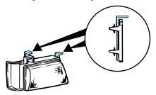
3. Disconnect the electrical connector from the bulb by pulling rearward.
