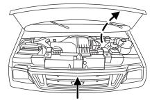
3. Lift the hood and secure it with the prop rod.
