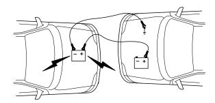
4. Make the final connection of the negative (-) cable to an exposed metal part of the stalled vehicle's engine, away from the battery and the carburetor/fuel injection system. **Do not** use fuel lines, engine rocker covers or the intake manifold as *grounding* points.
