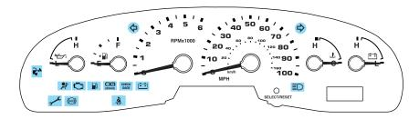
Warning lights and gauges can alert you to a vehicle condition that may become serious enough to cause expensive repairs. A warning light may illuminate when a problem exists with one of your vehicle's functions. Many lights will illuminate when you start your vehicle to make sure the bulb works. If any light remains on after starting the vehicle, have the respective system inspected immediately.
