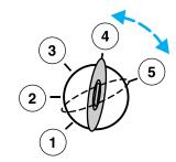
**Note:** If the engine does not start within five seconds on the first try, turn the key to 3 (OFF), wait 10 seconds and try again. If the engine still fails to start, press the accelerator to the floor and try again; this will allow the engine to crank with the fuel shut off in case the engine is flooded with fuel.
