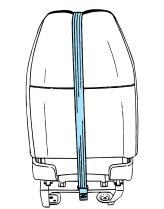
4. Clip the tether strap hook to the seat pedestal to the location shown.
