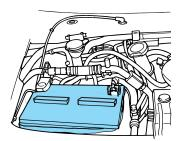
However, for severe usage or in high temperature climates and only for frame mounted deep cycle auxiliary batteries, check the battery electrolyte level. Note: This does not apply to production frame mounted or underhood batteries. Refer to the *Scheduled Maintenance Guide* for the service interval schedules.
