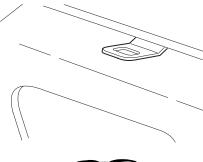
3. Route the child safety seat tether strap over the back of the front right-hand passenger seat as shown.
