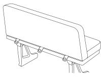
3. Clip the tether strap hook to the tether bracket mounted under rear rail of seat cushion frame.
