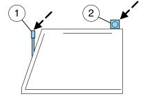
• **Sealed beam:** Locate the vertical adjuster (1) for each headlamp. Adjust the aim by turning the adjuster control either clockwise (to adjust up) or counterclockwise (to adjust down).
