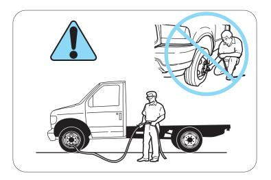
**WARNING** An inflated tire and rim can be very dangerous if improperly used, serviced or maintained. To reduce the risk of serious injury, never attempt to re-inflate a tire which has been run flat or seriously under-inflated without first removing the tire from the wheel assembly for inspection. Do not attempt to add air to tires or replace tires or wheels without first taking precautions to protect persons and property.
