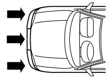
near-frontal collisions, not rollover, side-impact, or rear-impacts unless the collision causes sufficient longitudinal deceleration.
