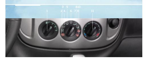
1 Fan Speed Control: Rotate the knob to adjust the speed of air that is circulated climate control system is turned off. in the vehicle.
