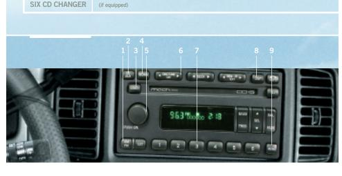
1 AM/FM and CD Select: In radio mode. press AM/FM to select AM or FM frequency bands. In CD mode, press AM/FM to stop play and begin radio play. To begin CD play control for five seconds; press the SEL while in radio mode, press the CD control.
