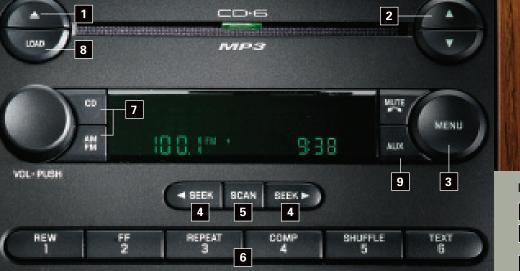
EJECTING CDS (CD EJECT): Press to eiect a CD. For In-dash CD6/MP3 system (if equipped), press and hold to auto-eject all CDs present in the system.
