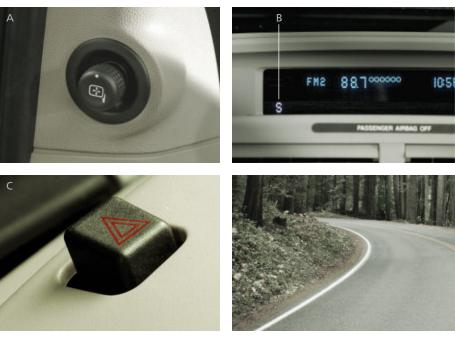
A. POWER SIDE VIEW MIRRORS – Rotate the control clockwise to adjust the right mirror, and counterclockwise to adjust the left mirror. Then move the control in the direction you wish to tilt the mirror. Return to the center position to lock the mirror in place.
