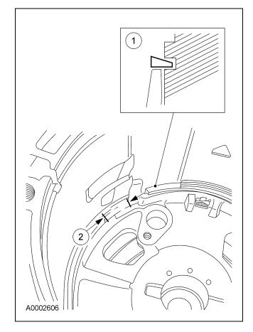
59. Install the center shaft thrust bearing (No. 3).
