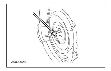
117. A CAUTION: The special tool must be used to correctly align the adapter plate to the converter or transmission damage could occur.
