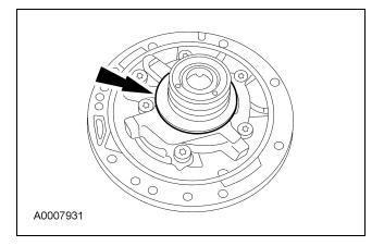
79. Install the special tools into the transmission case.
