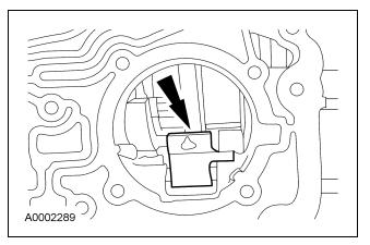
20. Install the reverse band actuating lever shaft into the case and into the reverse band actuating lever.
