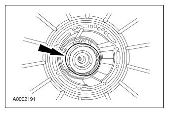
61. CAUTION: Do not bend the trigger wheel. Make sure that the No. 2 thrust bearing is in this assembly.
