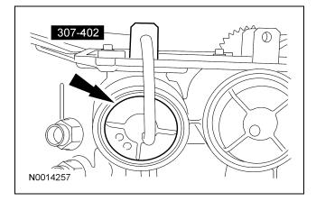
65. **NOTE:** If the overdrive band is reused, it must be installed in the same position as when removed.
