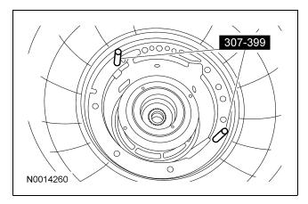
80. Install the pump gasket.
