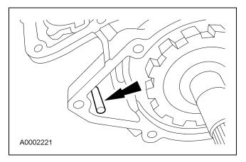
21. Install the No. 10 needle bearing into the case.
