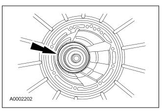
37. Install the No. 5 thrust bearing.
