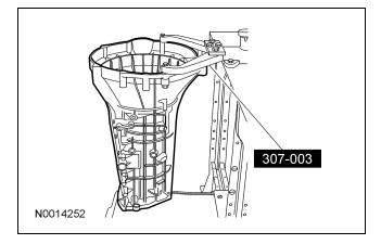
6. Using the special tool, install the manual control lever shaft seal and lubricate it with petroleum jelly.
