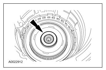
36. Install the forward clutch cylinder.
