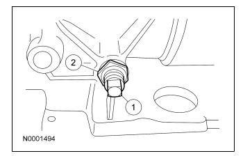
88. **CAUTION:** Do not allow the intermediate band adjusting screw to back out. Band strut could fall out of position.
