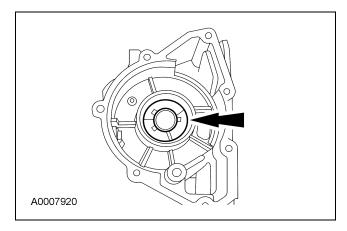
15. Install the park gear on the output shaft.
