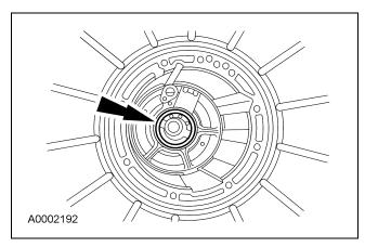
60. Install the overdrive ring gear, overdrive one-way clutch and center shaft assembly.
