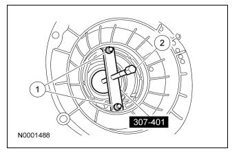
43. **NOTE:** Align the disc holes on special tool with the slot in gauge bar for correct measurement.
