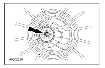
24. **NOTE:** Install the output shaft sleeve with the cone facing up. This sleeve will snap into place when correctly installed.
