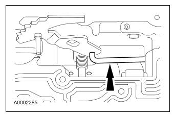
10. CAUTION: Align the flats on the manual valve inner lever with the flats on the manual control lever shaft.
