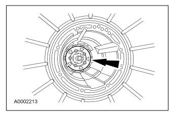
28. Install the No. 8 thrust bearing.
