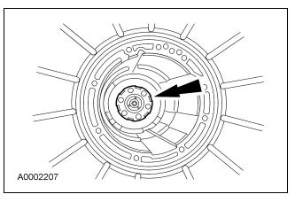
32. Install the No. 7 forward planet thrust bearing into the forward ring gear and hub assembly. Use petroleum jelly to hold the bearing in place.
