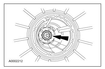
29. Install the spacer on the input shell, using petroleum jelly to hold it in place.
