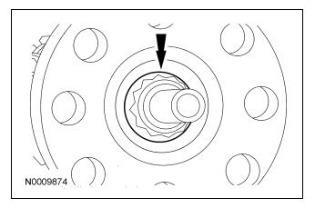
109. A CAUTION: The digital transmission range sensor must fit flush against the boss on the case to prevent damage to the sensor.
