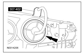
40. Install the direct clutch drum.
