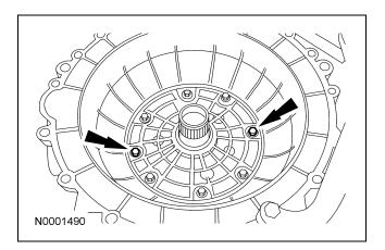
85. CAUTION: Do not allow overdrive band adjustment screw to back out. Band strut could fall out of position.
