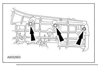
120. **NOTE:** Inspect O-ring seal for damage. Install new if damaged. Lubricate the O-ring seals with petroleum jelly to prevent damage to the O-ring seals.
