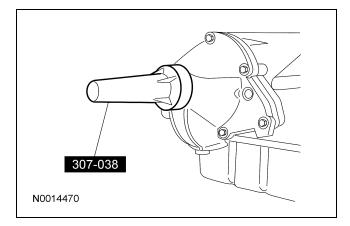
107. Using the special tools, install the output shaft flange.
