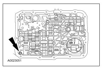
96. Tighten the screws in the sequence shown.
