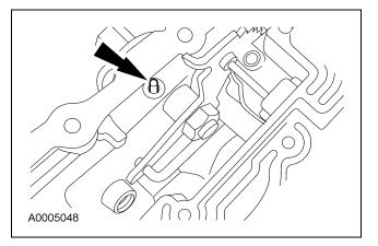
13. CAUTION: To avoid damage, do not allow the wrench to strike the manual valve inner lever pin.
