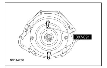
116. Lubricate the torque converter pilot hub with multi-purpose grease.
