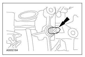
71. Install the overdrive apply strut.
