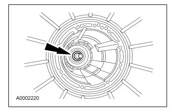
22. CAUTION: Do not damage the seal against the case during assembly.
