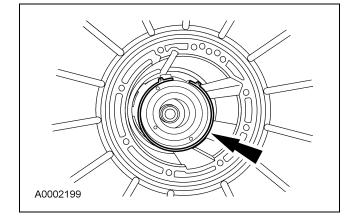
48. Install the intermediate band anchor strut.
