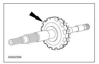
16. Install the output shaft and park gear.
