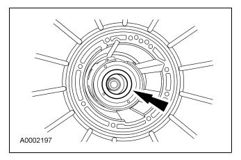
55. **NOTE:** Align the center support screw hole with correct case hole.
