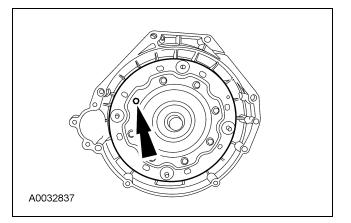
119. Using one of the speed sensor holes, fill the transmission with 8.5L (9 quarts) of automatic transmission fluid.
