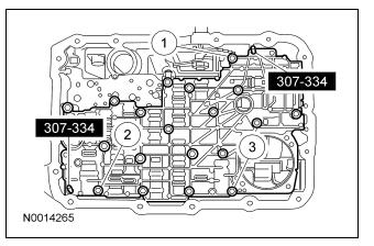
95. Remove the special tools, and loosely install the screw.
