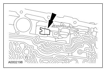
49. CAUTION: To avoid a "fall-out" condition of the strut from the screw during assembly and function, the small "U" shape notch should be toward the band/case side and the large "U" shape notch toward the main control side.
