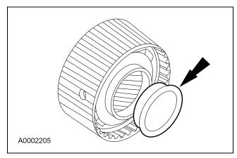
34. Install the forward ring gear and hub as an assembly.
