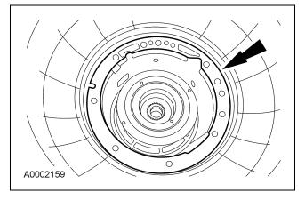
81. CAUTION: Make sure that the fluid pump inlet thrust washer (No. 1), selective thrust washer, fluid pump gasket and the fluid pump-to-case O-ring seal remain in the correct position throughout this step.
