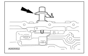
11. Install the manual valve inner lever onto the manual shaft and loosely install the nut.
