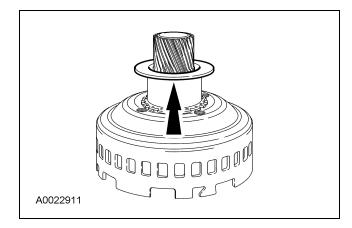
30. Install the input shell and sun gear assembly.
