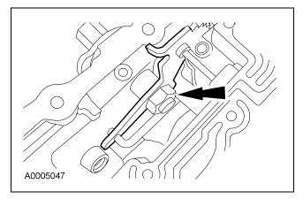
12. CAUTION: Use care not to damage the fluid pan rail surface when installing the retaining pin.
