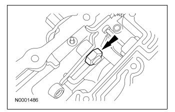
14. CAUTION: The tabs on the output shaft thrust washer (No. 11) point into the case. Make sure the thrust washer is correctly seated.
