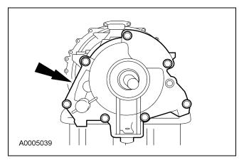
106. Using the special tool, install the extension housing seal.
