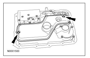
102. **NOTE:** The transmission fluid pan gasket is reusable. Clean and inspect for damage. If not damaged, the gasket should be reused.
