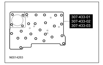
93. Install the special tools into the transmission case.
