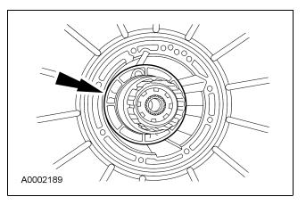
62. Install the overdrive brake drum and coast clutch drum assembly.
