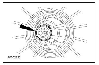
18. CAUTION: Make sure band is resting on the 2 anchor pins in the case.
