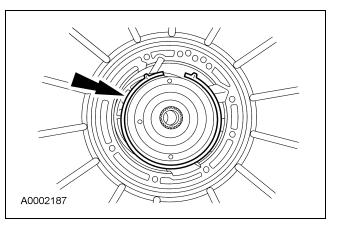
66. Install the overdrive anchor strut.
