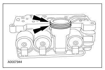
99. CAUTION: Inspect the transmission case bore to make sure it is free of debris and not damaged. If damaged, transmission leak may occur.
