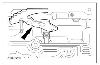
9. Assemble the manual valve inner lever and parking lever actuating rod as shown.
