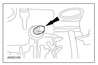
52. Install the intermediate band apply strut.
