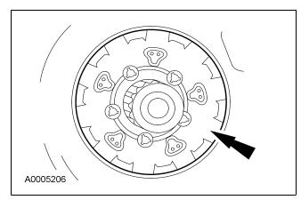
27. A CAUTION: The low/reverse brake drum must be pulled forward to install the low/reverse planet retaining ring.
