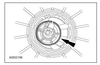
56. Install the center support locknut and cage.
