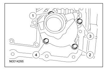
101. CAUTION: Lubricate the fluid filter seals with clean automatic transmission fluid or they may be damaged.
