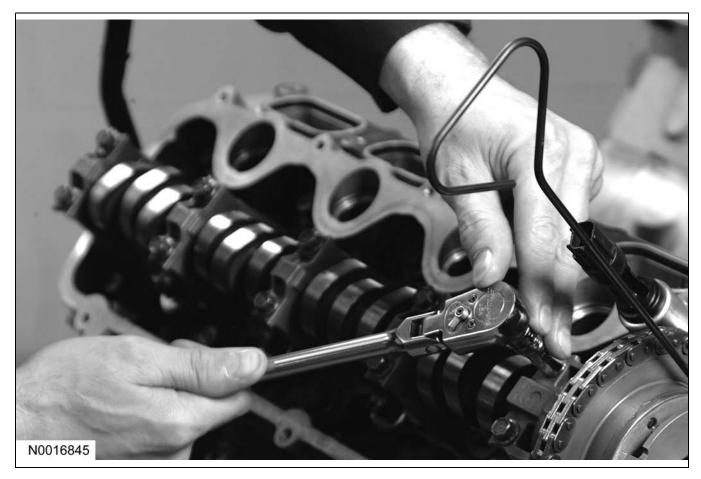
Loosen #1 Camshaft Bearing Cap Bolts
