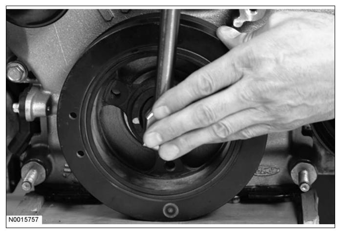
Set Crankshaft Damper Spoke to 6 o'clock Position
