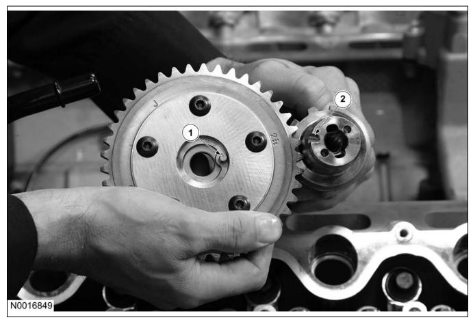
Phaser Pin and Cam Notch
