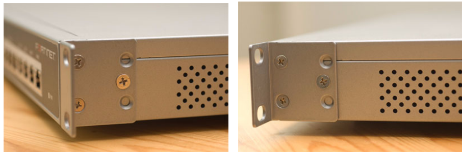
Figure 2: Installed mounting brackets
