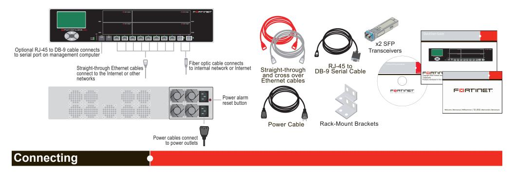
Connect the following to the FortiGate unit. Ensure the FortiGate unit is placed on a stable surface or install in a standard 19 inch rack.
