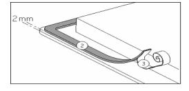
Stick the gasket (2) two millimeters from the external edge of the glass, after removing the protection sheet (3).
