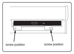
Use the screw you removed in step 1 to fix the blank panel supplied with the CD-1A to the front panel.
