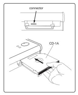
3 Use two screws supplied with the CD-1A to fix the CD-1A to the VF160 from the front panel. Tighten the screws with a screwdriver.
