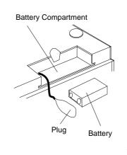
Open the mixer bottom battery compartment lid by hand, correctly connect the plug to the battery, and place battery in compartment and replace lid as before.
