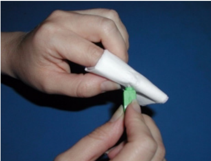
Figure 19 Wiping the connector with a Kim wiper
