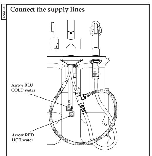
Connect the hot and cold supply lines. Do not allow the supply tubes to twist or bend sharply. Leave the valves closed.
