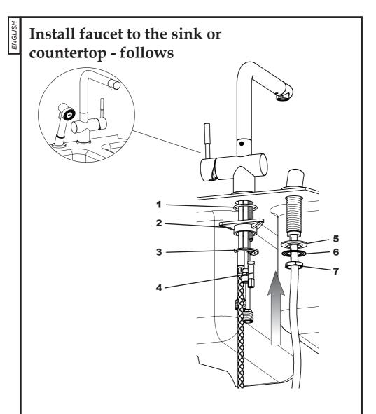
Install the fastening components to the faucet's threaded shank in the following sequence: round gasket (1), triangular flange (2), metal washer (3) and threaded nut (4) (the triangular flange can be omitted if the sink/countertop is too thick). Install the fastening items of the spray head holder in the following sequence: the flat rubber washer (5), the metal washer (6) and the threaded nut (7).
