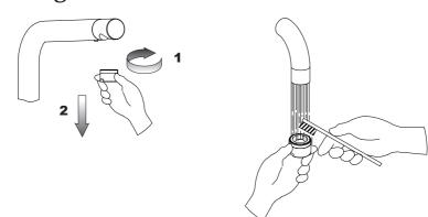
It is recommended that you periodically clean the aerator of your faucet. To do so, unscrew the aerator holder from its own seat. Simply using a toothbrush, or something similar, rub the filter under the water, removing the impurities and any build up. Screw the areator back into place.
