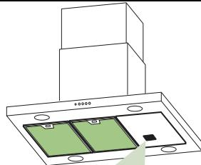
Connect the extractor to the exhaust flue through a pipe of minimum diameter 120 mm. The route of the flue must be as short as possible.
