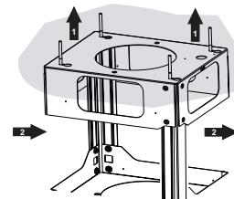
Before tightening the screws completely it is possible to adjust the frame by turning it. Make sure that the screws do not come out of their seats in the slotted holes.
