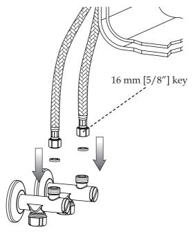
Connect the supply line. In order to guarantee a long use of the product, install the angle valve equipped with filter and clean them regularly. Do not allow the supply tube to twist or bend sharply.
