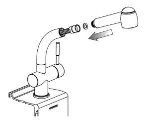
Attach the pull-out spray head to the hose.
