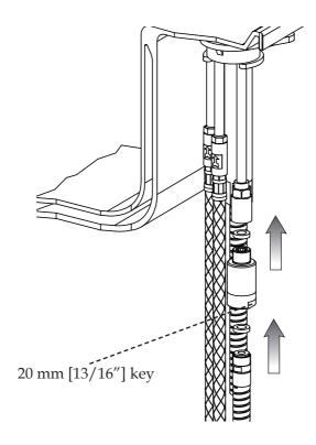
Attach the valve-holder to the shorter tubing and attach the spray hose to the valve-holder.
