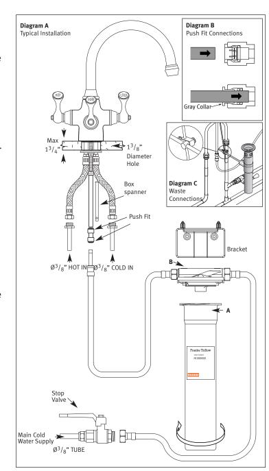
**9** For optimum filter performance use the stop valve to set the filtered water flow to  $2^{3/4}$  -  $3^{1/2}$  pints/min (1  $^{1/2}$  - 2liters/min).
